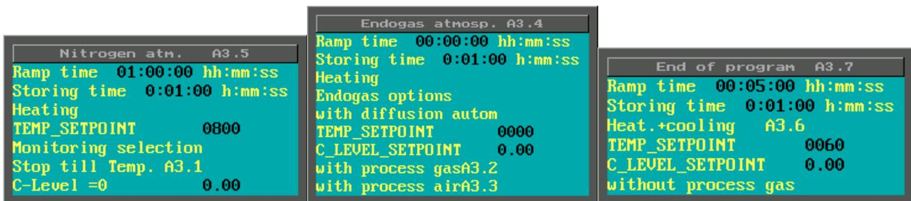
Fig. 6: Set points of the single program sections
