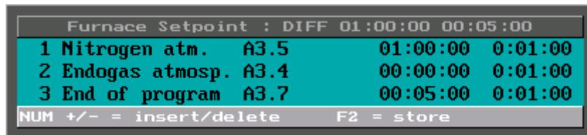
Fig. 5: Example for sections of a program
