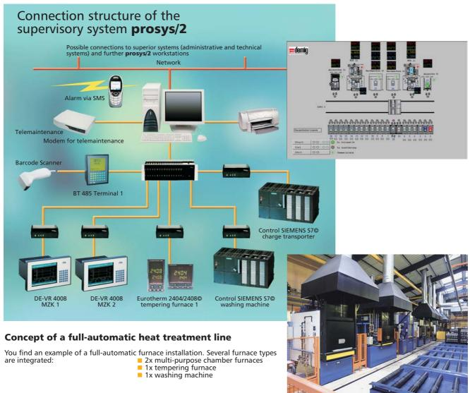
The furnaces are charged by means of a charge transporter which works according to the instructions of **prosys/2**. The login and logout will be effected by the terminal.
